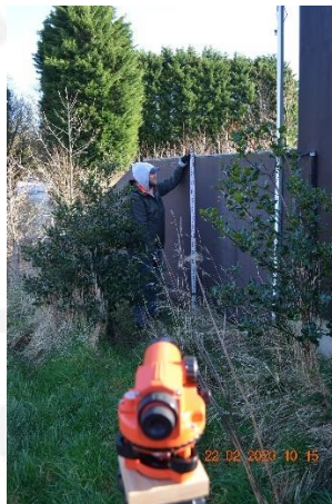
228 229 Figure 5: view of the transit and survey pole. One individual operated the transit while the other steady the survey pole to 230 record a measurement.
