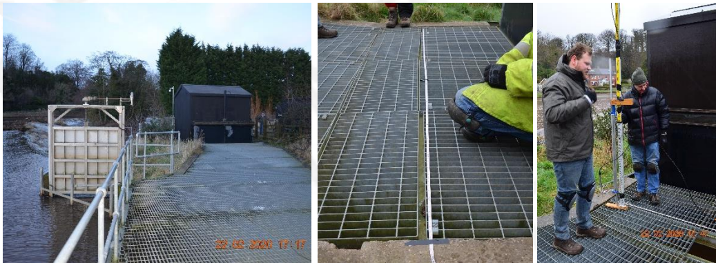
264 265 Figure 7: view of sluice gate and flow measurement area from the upstream opening of the inlet channel (left, a), measuring 266 tape placed along the inlet channel's cross-section to measure velocity and known horizontal locations (middle, b), and two 267 individuals with the Sontek ADV ® sensor and extended pole ready to measure flow velocity through an open inlet channel 268 grate (right, c).
