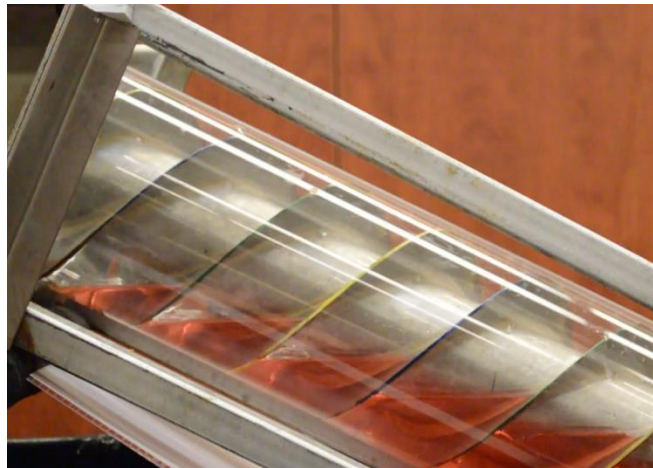
Fig. 3. Fill height gradient as observed experimentally.
