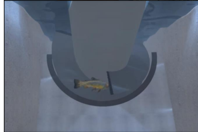
Coarse intake grate allows passage of fish and small debris. (Greenbug Energy Inc., 2012)
