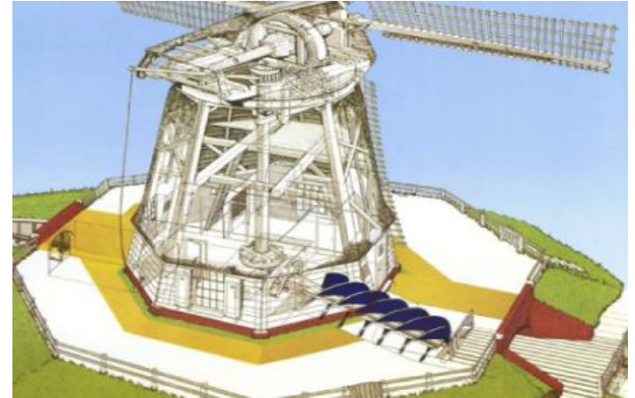
Archimedes screw pump in a Polder Mill (Greenbug Energy, 2016).
